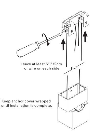
When desired height and level are achieved, tighten the strain reliefs.
