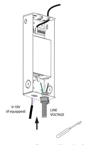
Use a screwdriver to knock out tab, then secure cables (not provided)
