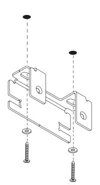
Install anchor strain relief. Make sure nylon set screw is facing the outside of the bracket.
