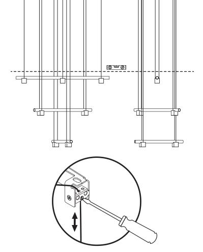
Make sure all the cubes and slabs align with the anchors. They may have shifted with assembly and lead to
