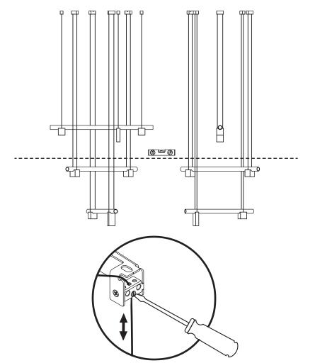
Make sure all the cubes and slabs align with the anchors. They may have shifted with assembly and lead to
