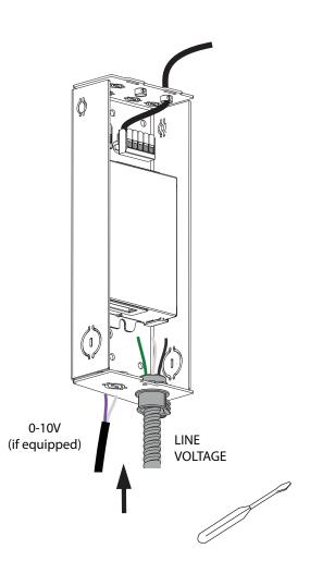
Use a screwdriver to knock out tab, then secure cables (not provided)
