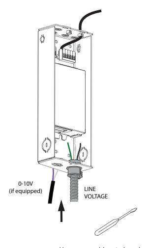
Use a screwdriver to knock out tab, then secure cables (not provided)
