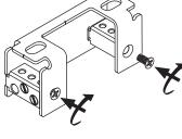
Install ceiling brackets. Strain relief side faces the electrical block anchor. strain relief Ø >OR β þ Y Cummer (3 **Q**\_0 බ mmme (3 æ mmmer (} \*use appropriate anchors
