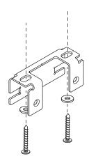
**Electrical side** Closed side of the bracket facing the canopy.
