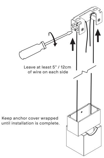
When desired height and level are achieved, tighten the strain reliefs.
