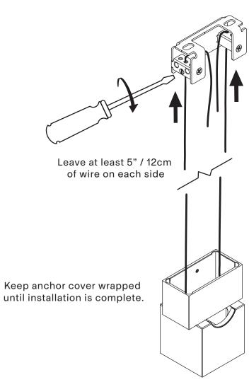
When desired height and level are achieved, tighten the strain reliefs.
