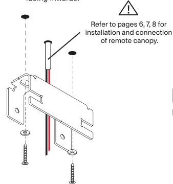
Non-electrical side Closed side of the bracket facing inwards.
