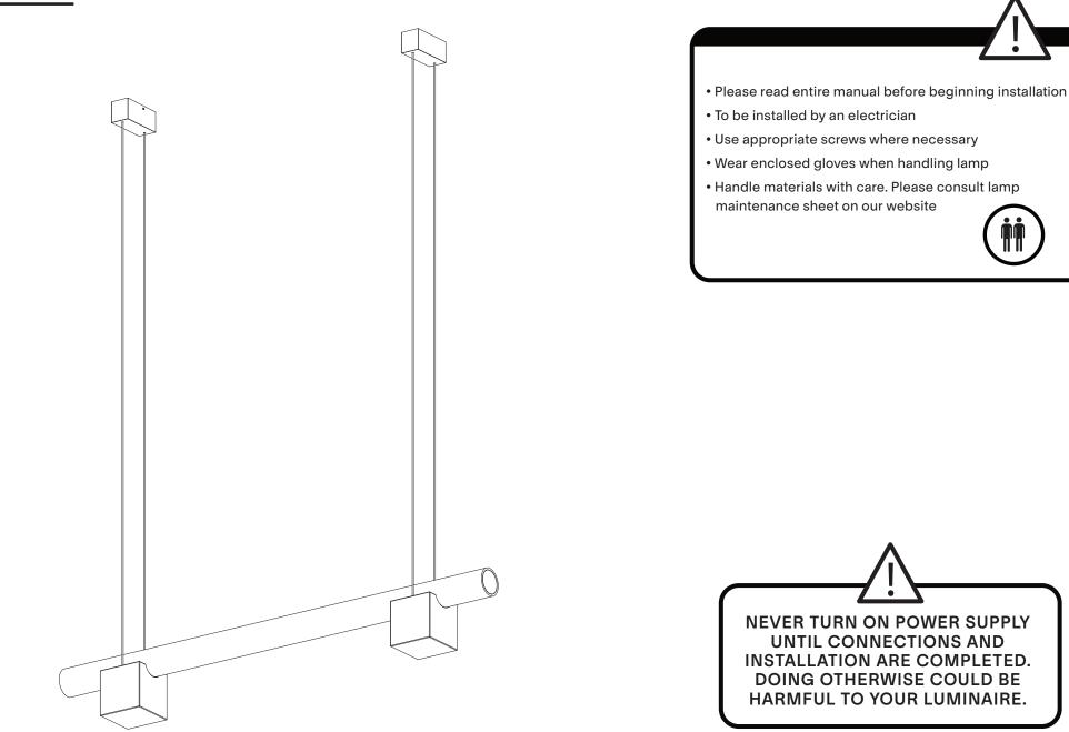
Mark anchor points. Make sure electrical wire will exit in M1 ceiling bracket.
