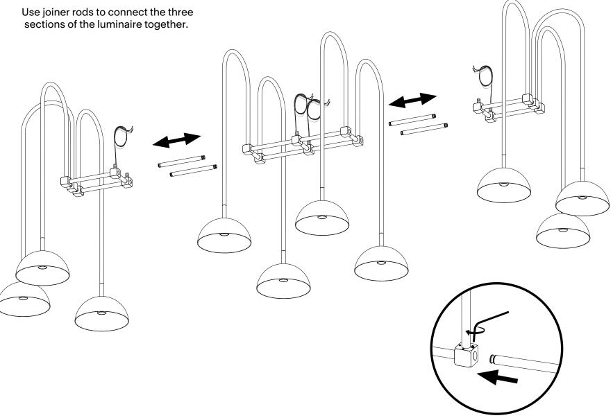
Insert joining rods, then tighten set screw gently, but firmly.
