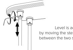
Level is adjusted by moving the stem up and down between the two segmented lines
