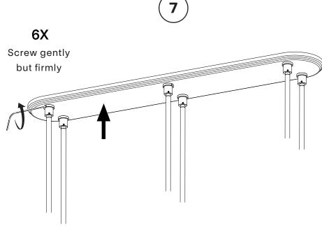
Ensure no wires are clipped or pinched during this operation.
