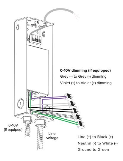
Use a screwdriver to knock out tab, then secure cables (not supplied)
