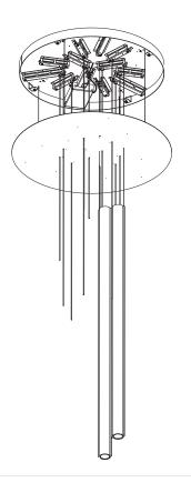
18" minimum  $\odot$ Ø Keep luminaires wrapped until the end of the installation
