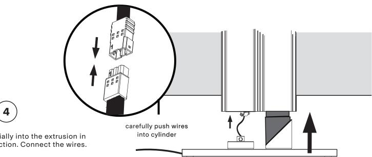
Push the weight partially into the extrusion in order to make connection. Connect the wires.
