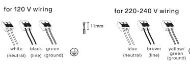
If applicable, use grey and purple wires for 0-10V dimming circuit, or the orange wires for DALI dimming circuit before closing the driver enclosure.
