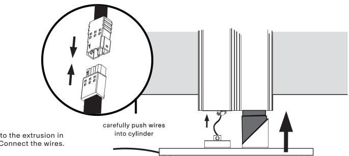
Push the weight partially into the extrusion in order to make connection. Connect the wires.
