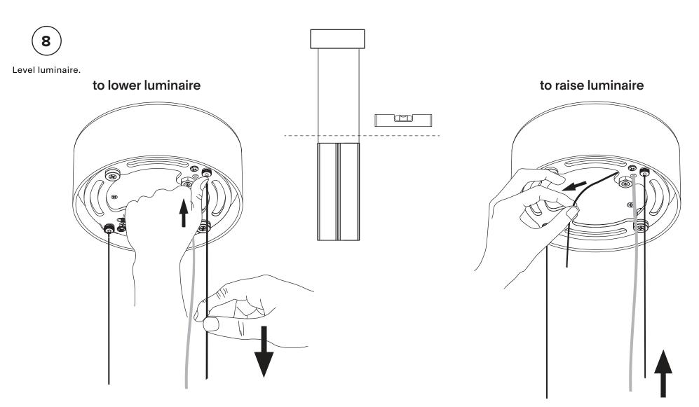
Losen lock, make adjustments as required, retighten lock.
