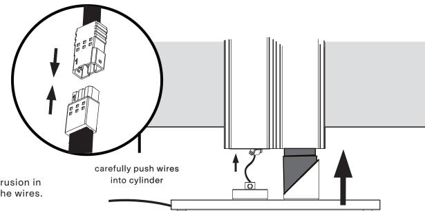
Push the weight partially into the extrusion in order to make connection. Connect the wires.
