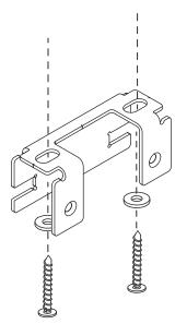
Electrical side Open side of the bracket facing the canopy.
