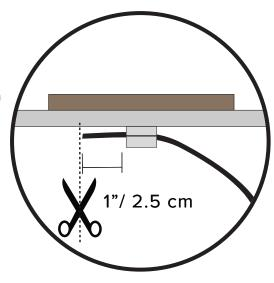
The extremity of the trimmed ribbon can be melted with the flame of a lighter for a few seconds to prevent fraying.
