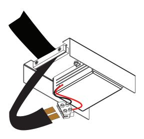
Both slots are the same and will receive either ribbon. (Polarity is not important)
