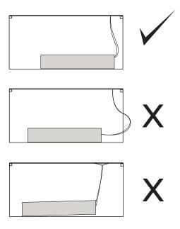
If your wires are too short or too long, unscrew end cap, losen strain relief screws on, pull wires out further while making sure the protective sleeve stays under the strain relief.
