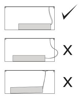
If your wires are too short or too long, unscrew end cap, losen strain relief screws on, pull wires out further while making sure the protective sleeve stays under the strain relief.
