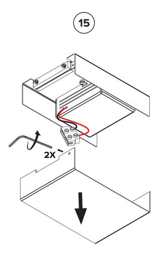
Remove the screws in the front and back of the canopy cover and lower it.
