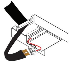
Both slots are the same and will receive either ribbon. (Polarity is not important)
