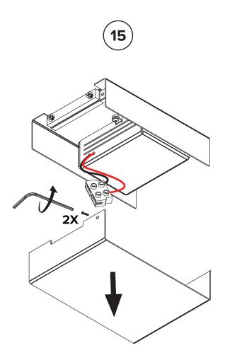
Remove the screws in the front and back of the canopy cover and lower it.
