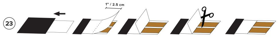
Push back the ribbon to reveal the copper conductor.
