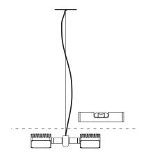
Moving the hex key will shift the lamp body left or right in order to balance it.
