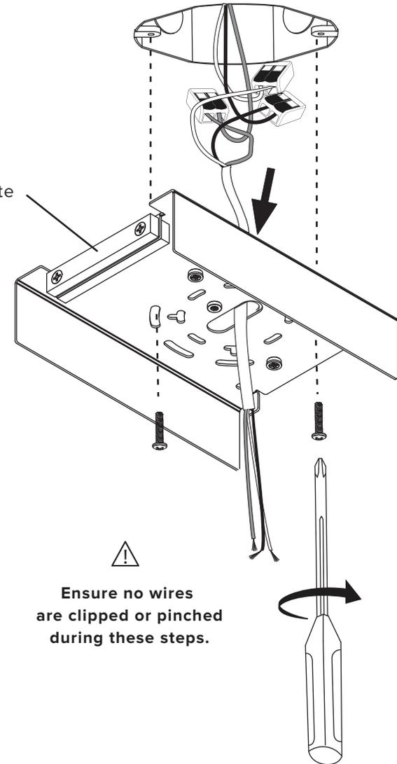
Ensure no wires are clipped or pinched during these steps.
