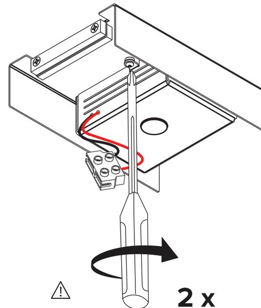
Ensure no wires are damaged during these steps.
