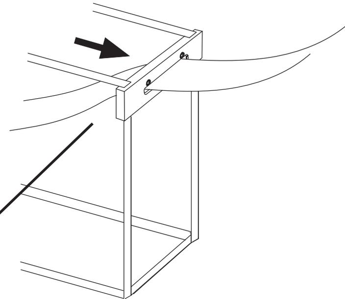
Pull ribbon until the glass shade is centered in between the two positioning threads. The wires should be approximately 2"/5cm from the edge of the glass.
