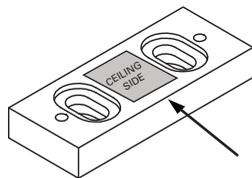
Note the ceiling side of the anchor is clearly labelled with a sticker.
