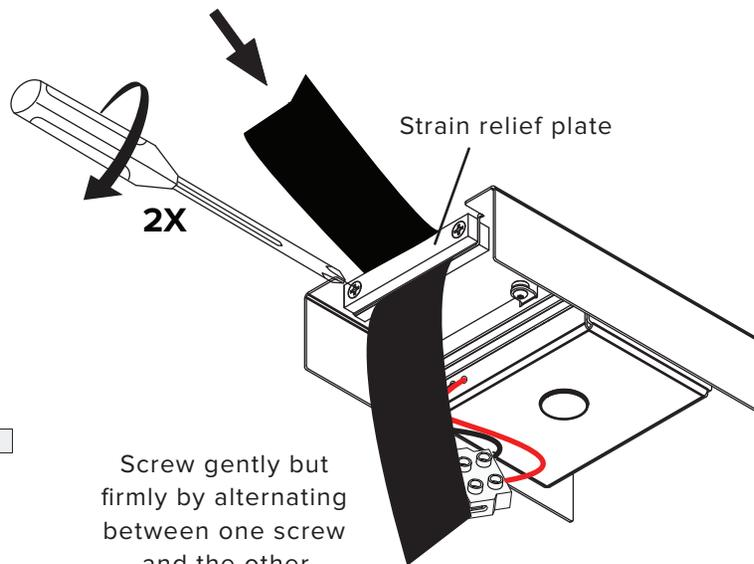
Screw gently but firmly by alternating between one screw and the other.
