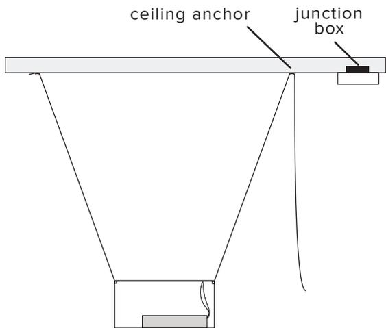
Insert the ribbon through the strain relief plate. Pull it down until the arc in between ceiling anchor and canopy is judged satisfying, then secure ribbon with the strain relief plate.
