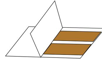
Fold the copper conductors in half onto themselves.
