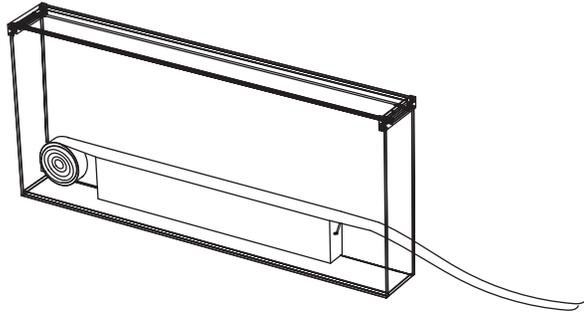
Pass both ribbons through the glass anchor system. Make sure there are no twists in the ribbon.
