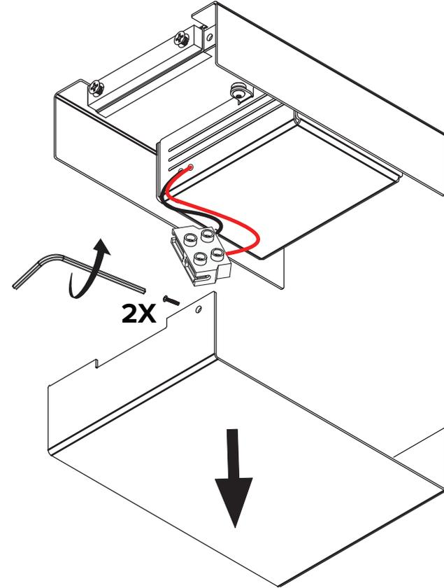
Remove the screws in the front and back
