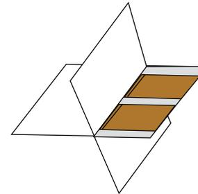
Trim off both white protective sheets. Then carefully cut between both conductor strips.
