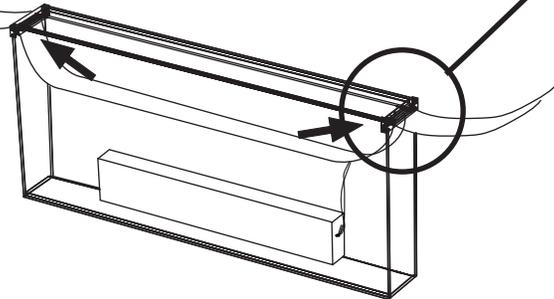
Pull ribbon until the glass shade is centered in between the two positioning threads. The wires should be approximately 2"/5cm from the edge of the glass.
