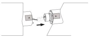
Align connector pin and push arms together
