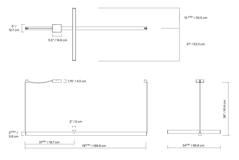
FINISH LAMP ANATOMY MR ΒK WН Polished Textured Textured ANCHOR aluminum black white NOTES CANOPY - Must be installed by an electrician - Not protected against liquids (refer to IP20) Additional charges for modifications or for special orders
