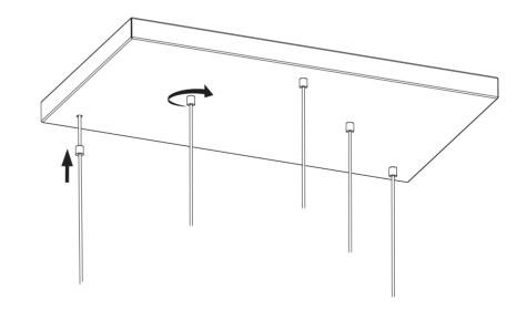
When adjustements are complete, raise the canopy cover and secure it in place by screwing the caps back into place.
