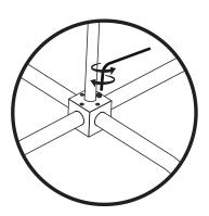
Losen set screw, resposition arm then tighten set screw gently, but firmly.
