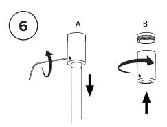
Loosen set screw and lower celing rod to allow mount to be screwed into the ceiling anchor
