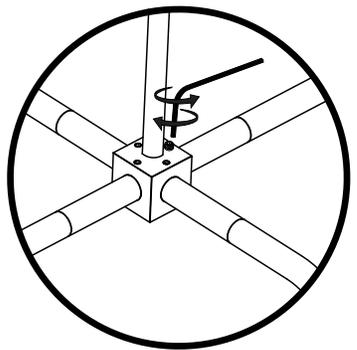
Loosen set screw, reposition arm then tighten set screw gently, but firmly.
