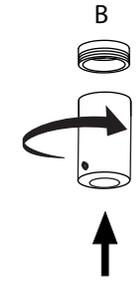
Loosen set screw and lower ceiling rod to allow mount to be screwed into the ceiling anchor
