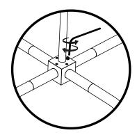
Losen set screw, resposition arm then tighten set screw gently, but firmly.
