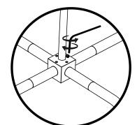
Losen set screw, resposition arm then tighten set screw gently, but firmly.
