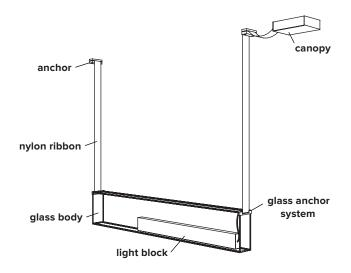
COLOUR NYLON RIBBON CANOPY **TEMPERATURE (CCT)** CONTROL top BK black warm light (2700K) 0-10V dimming (120V only) BK black WL ZΤ side B side A WH white NL neutral light (3000K) PH phase dimming DALI (220-240V only) DA D27 dim to warm (2700K to 2200K) bottom D30 dim to warm (3000K to 2200K) ССТ Other CCT available upon request\* WL BK BK ZΤ = STE06PLGRBKBKWLZT
