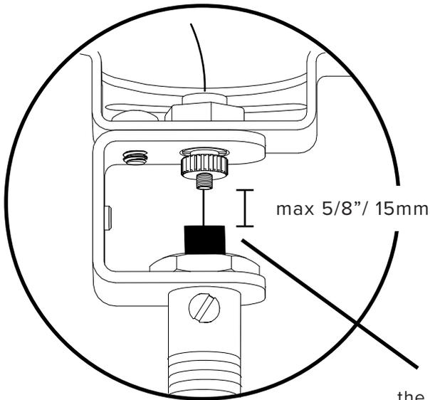
The sleeved section of the cord should be as close to cable gripper as possible.
