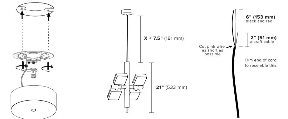
Ensure your electrical box can hold the weight of the luminaire (15 lbs) and that no wires are pinched during these steps.
