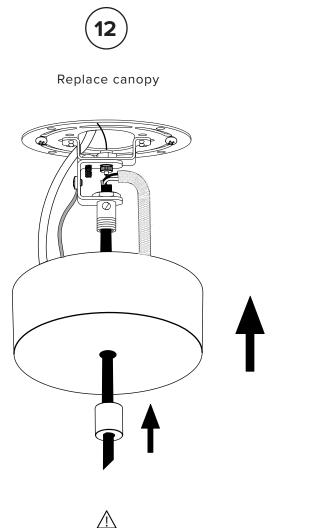
Ensure no wires are clipped or pinched during these steps.
