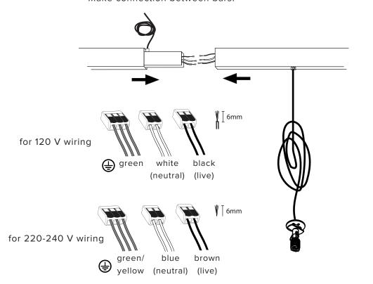
Carefully place wires and Wagos in between connecting plates of the bars before sliding the bars together.
