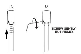
Raise ceiling stems into the anchored ceiling mount and tighten the set screw
