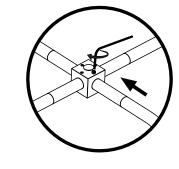
Insert removed arms into the cubes and secure set screws. The arms will be repositioned properly once the fixture has been installed to the ceiling.
