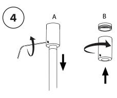
Loosen set screw and lower celing rod to allow mount to be screwed into the ceiling anchor
