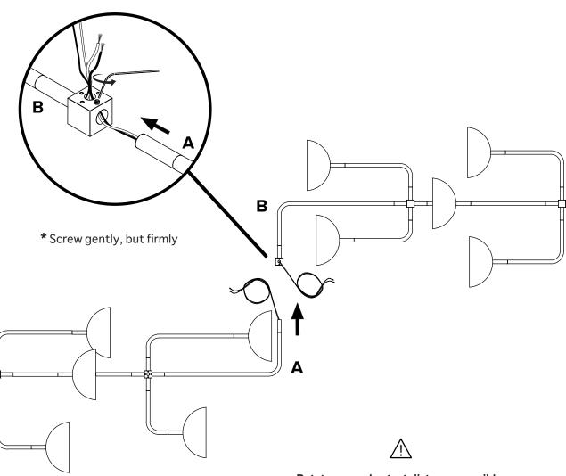
Rotate arms shortest distance possible. Do not rotate 3/4 turn.
