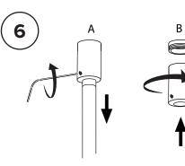
Loosen set screw and lower celing rod to allow mount to be screwed into the ceiling anchor
