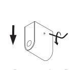
Remove or install cover by screwing and unscrewing set screw
