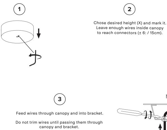
Leave ±6" / 15 cm of wire after strain relief to make connections. Leave 1"/ 2.5cm of sleeved wire after strain relief.
