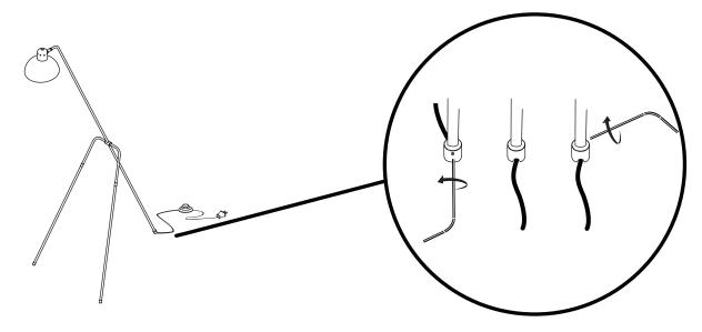
When the back leg has been screwed into place, rotate coupling so that the wire exit hole faces back from the lamp. Losen set screw before adjusting and tighten it again when finished.
