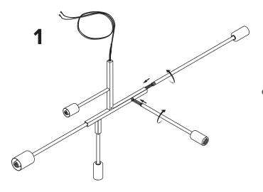
Rotate each arm 5 full rotations counterclockwise before inserting arms into body to prevent wires from over twisting.
