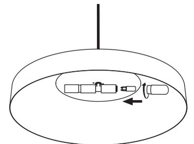
Ensure no wires are clipped or pinched during this operation.
