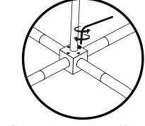
Losen set screw, resposition arm then tighten set screw gently, but firmly.
