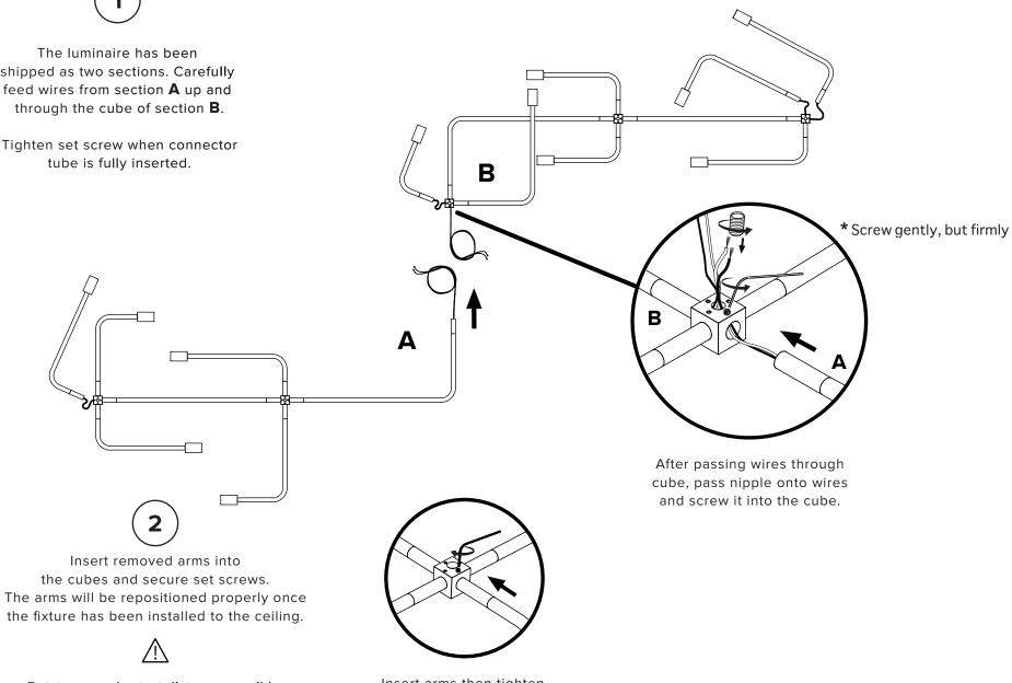
Rotate arms shortest distance possible. Do not rotate 3/4 turn.
