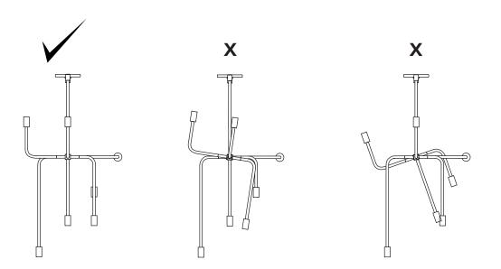
B Vertical level is adjusted by moving the stem up and down between the two segmented lines
