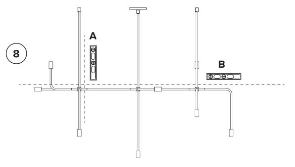
Horizontal level is adjusted by tightening and losening the ceiling mount screws.
