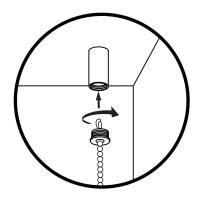
Adjust chain lenghts before installing them to the ceiling. When luminaire is level trim excess cable
