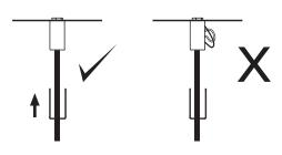
Ensure no wires are clipped or pinched during this operation.
